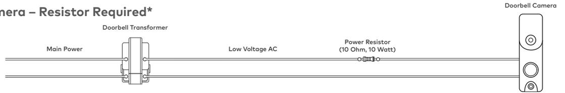
**WARNING:** This setup is designed for testing and demonstration purposes only. Failure to install a resistor (10 Ohm, 10 Watt) when a chime is not present may result in damage to the doorbell camera.
